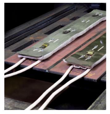
Measure the preheat temperature here 75 mm Intended weld joint
