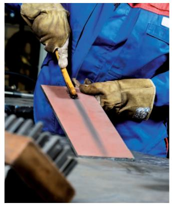
Welding can be carried out directly on the excellent Weldox and Hardox primer, due to its low zinc content.
