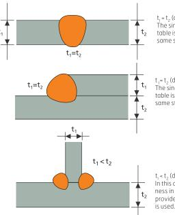
t<sub>1</sub> = t<sub>2</sub> (dimensions in mm) The single plate thickness in the table is  $t_{_{\rm I}}\,{\rm or}\,t_{_{\rm 2'}}$  provided that the same steel type is used.
