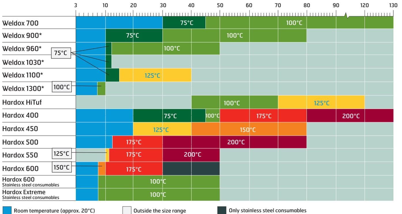
Note: The table is applicable to single plate thickness when welding with a heat input of 1.7 kJ/mm. Further information on single plate thickness can be found in TechSupport #61 at [www.ssab.com](http://www.ssab.com).
