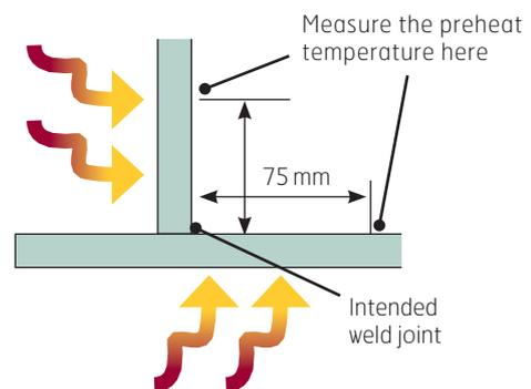
Measure the temperature of the thickest plate in the joint. If the plate is 25 mm thick, measure the temperature 2 minutes after heating. If the plate is 12.5 mm thick, measure the temperature after 1 minute, etc. The interpass temperature can be measured in the weld metal or in the immediately adjacent parent metal.
